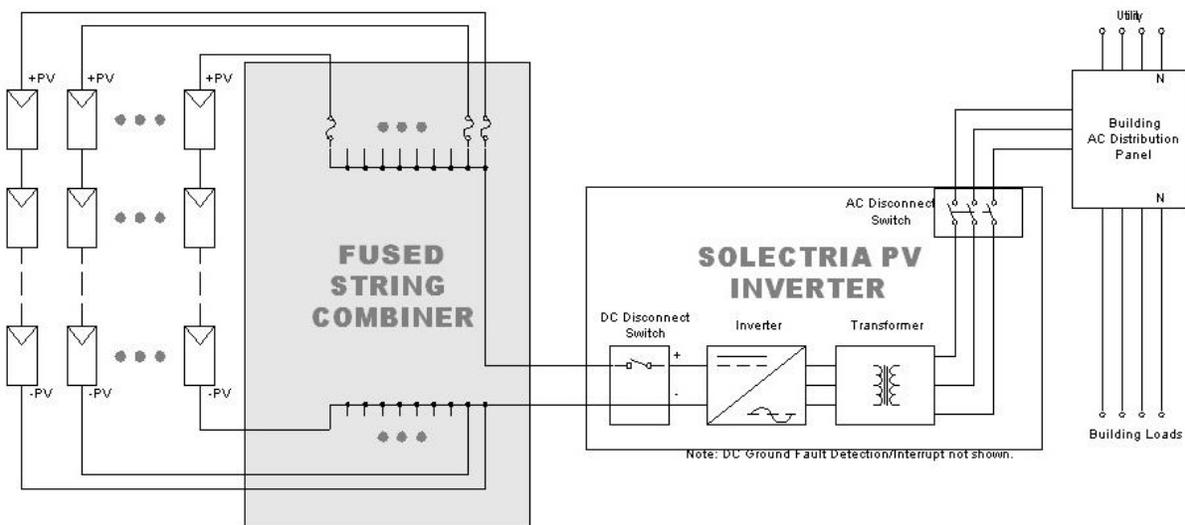
**Fig. 3 Simplified electrical connection diagram**
