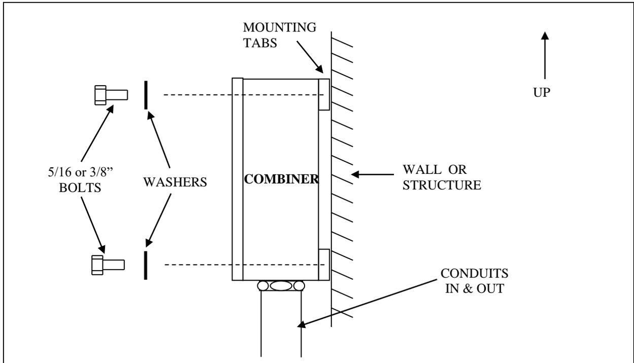
**Fig. 2b STRCOM Fused Combiner Mounting Diagram (side-view)**
