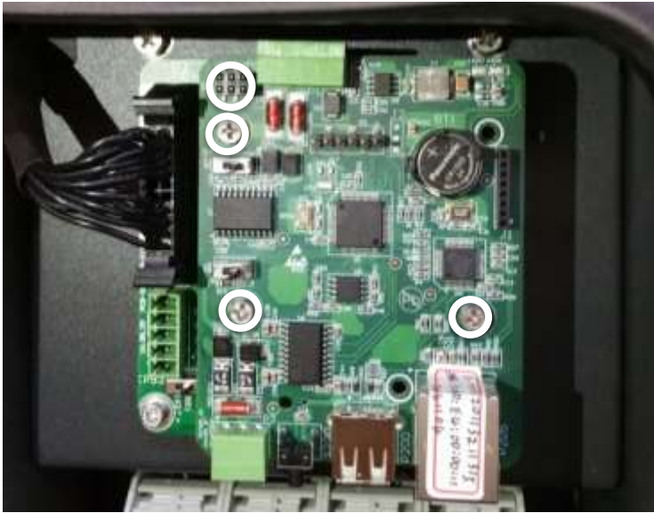
Figure 2-3 Ethernet Network card installed
