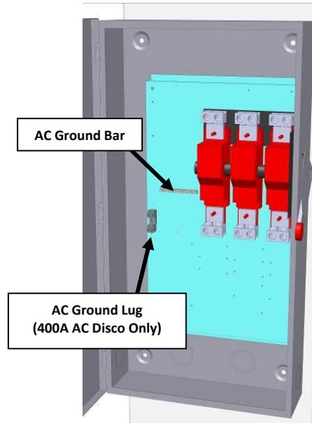
**Fig. 4.1b AC Ground Connection – 400A
