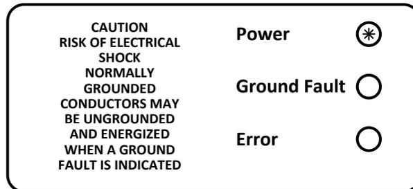
Figure 1 – LED Indicators displaying Normal Operation (green)
