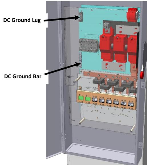
**Fig. 4.2 DC Ground Connection
