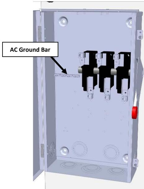
**Fig. 4.1a AC Ground Connection – 200A
