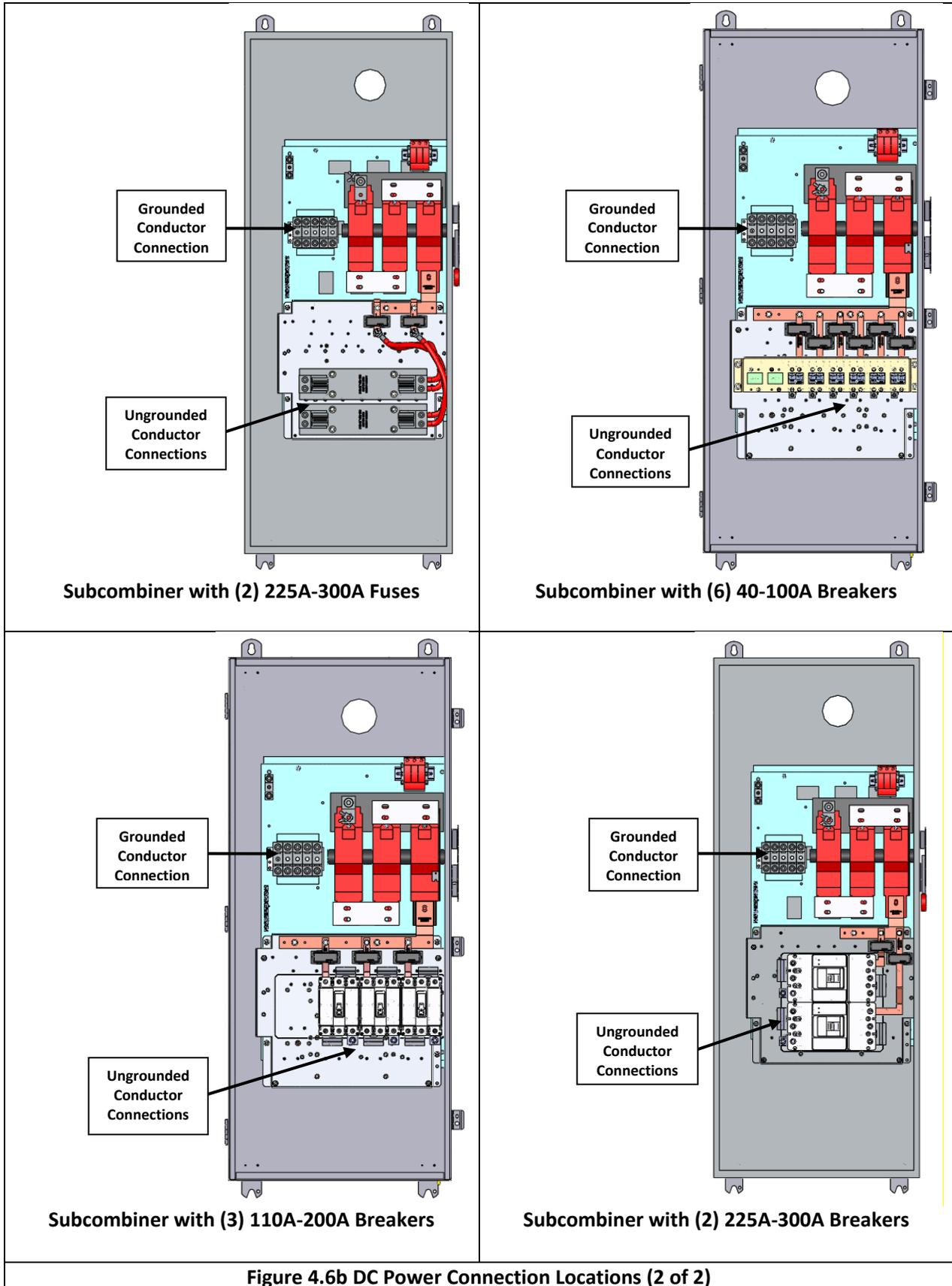
Figure 4.6b DC Power Connection Locations (2 of 2)
