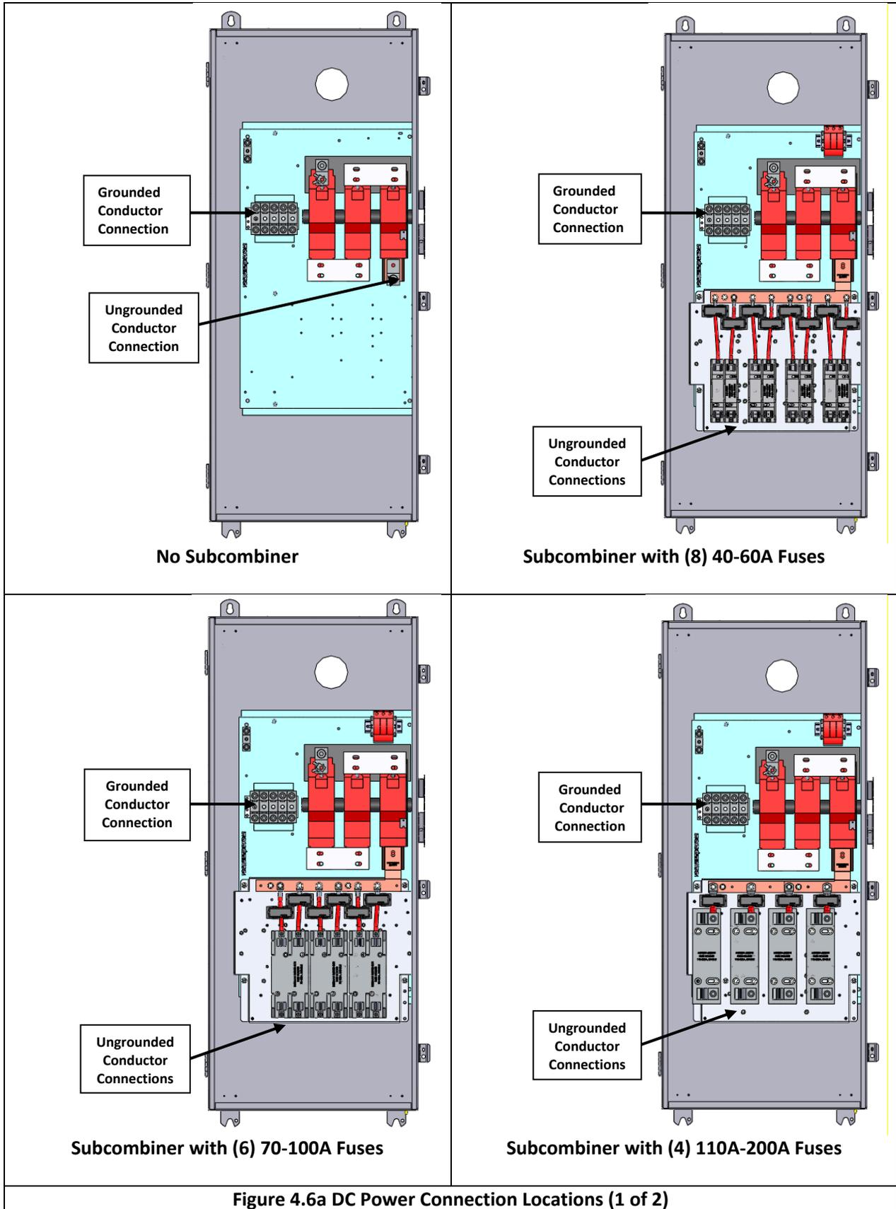
Figure 4.6a DC Power Connection Locations (1 of 2)
