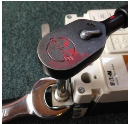
**Figure 4.7 – Lug Damage Prevention**
