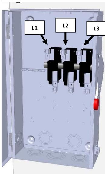
**Fig. 4.3 AC Power Connections - 200A
