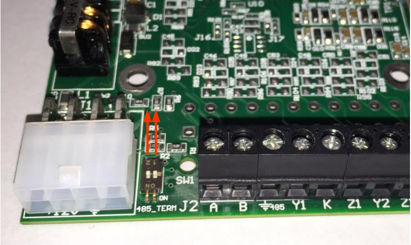
Figure 2.41b - The SolrenView Data Logger Printed Circuit Board and the Modbus Termination Dip Switches. Rev 4 or newer board.
