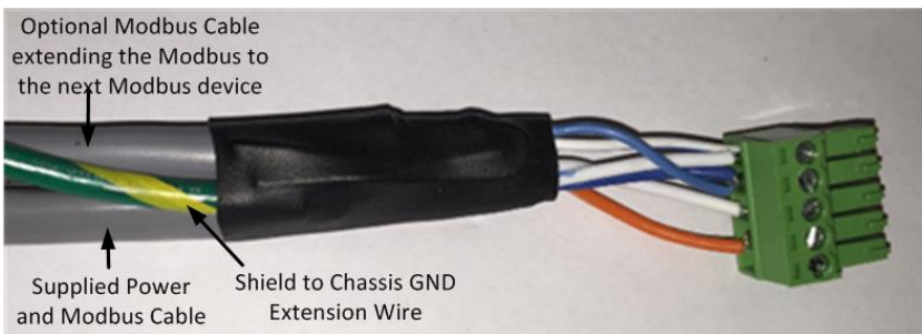
Figure 2.42 - Close up showing how the SolrenView Data Logger power and Modbus cable, the shield extension, and the optional Modbus cable extension connected to the P208 connector terminal block. Don't expose any more than 2" of wire outside of the shield.
