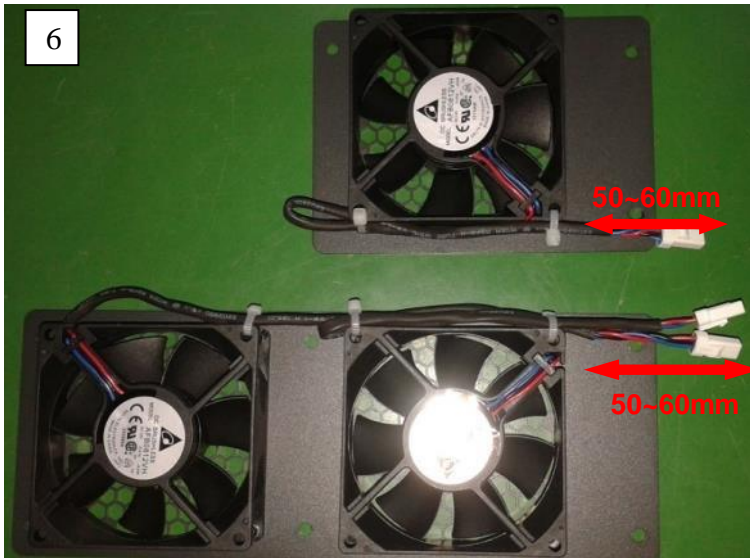
Figure 6.1 - Replace Cooling Fans
