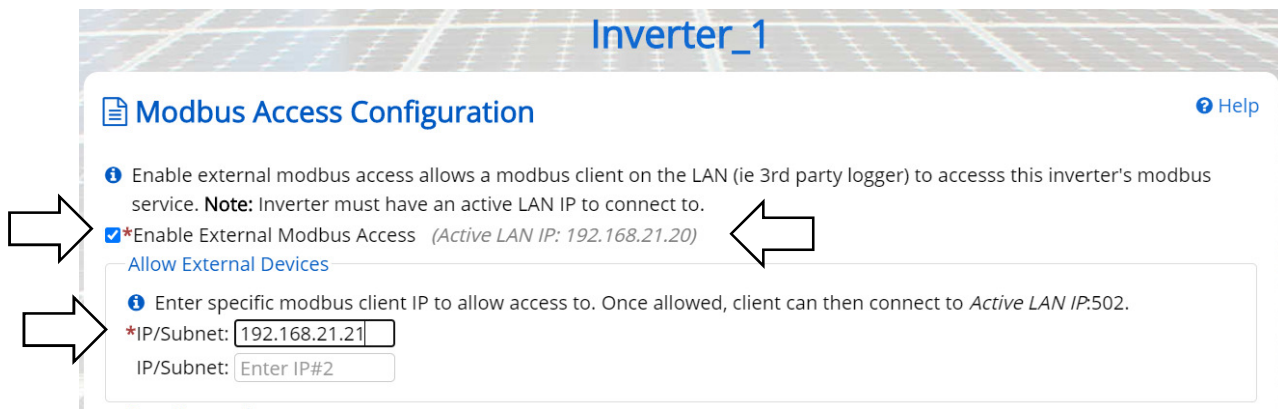
Figure 5-6 Enabling external Modbus access, Port Forwarding
