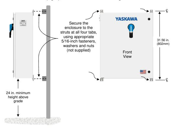
Figure 4.2 - CR1500-xxP Combiner example mounting to struts
