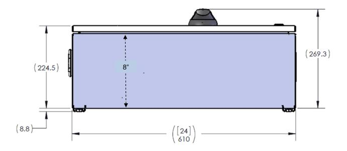
Fig 4.3 Bottom of the CR1500-xxP Enclosure
