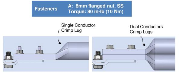
Figure 4.5 – Compression Lug Connections, Single and Dual Conductors
