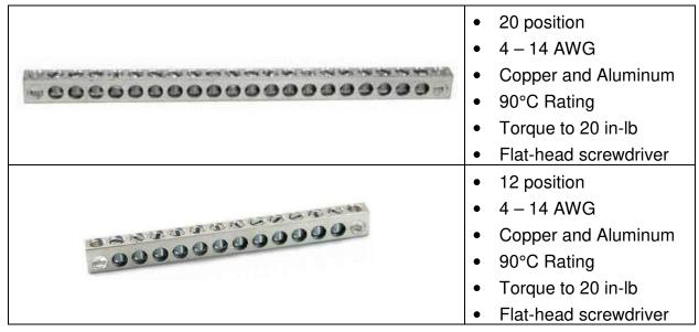
Fig. 4.6 - PV Source Circuit Equipment Ground Terminals
