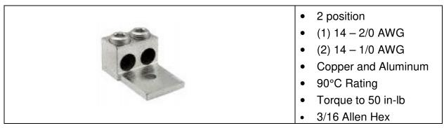
Fig. 4.7 - PV Output Circuit Equipment Ground Terminal
