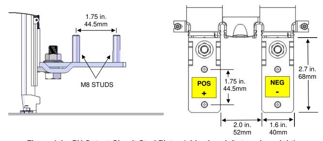
Figure 4.4 – PV Output Circuit Stud Plates (side view, left; top view, right)
