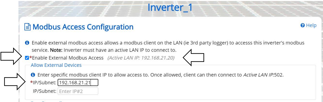
Figure 5-6 Enabling external Modbus access, Port Forwarding
