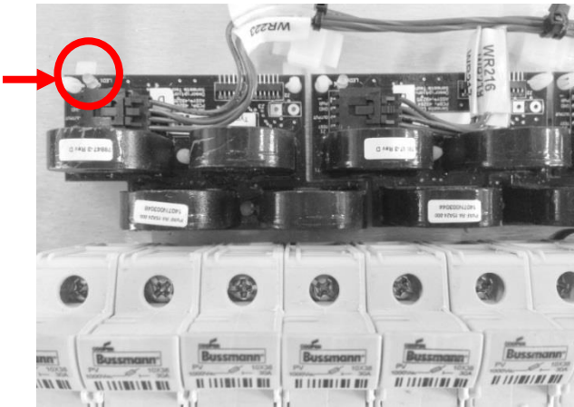
Picture 6 – Arc Sensing Boards and LED Indicators
