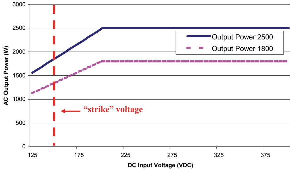
Fig. 11 AC Output power of PVI 1800/PVI 2500
