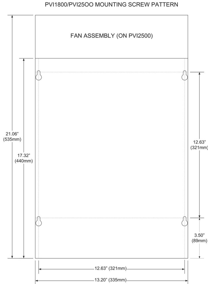
**Fig. 5 PVI 1800/PVI 2500 Mounting Screw Pattern**
