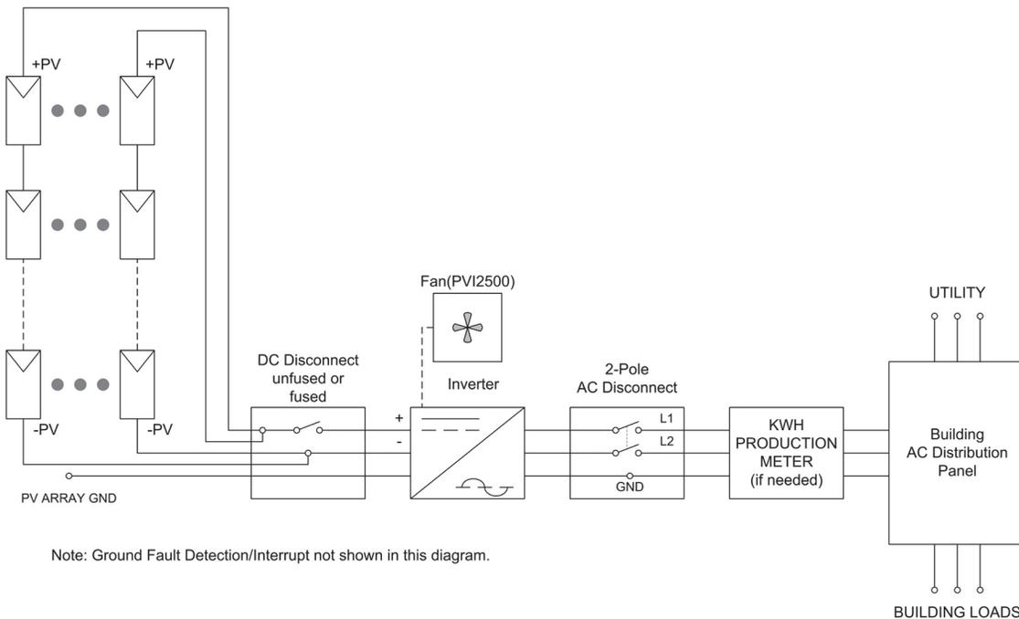
**Fig. 6 Simplified electrical connection diagram**
