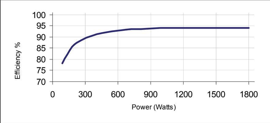
Fig. 13a PVI 1800 efficiency plot
