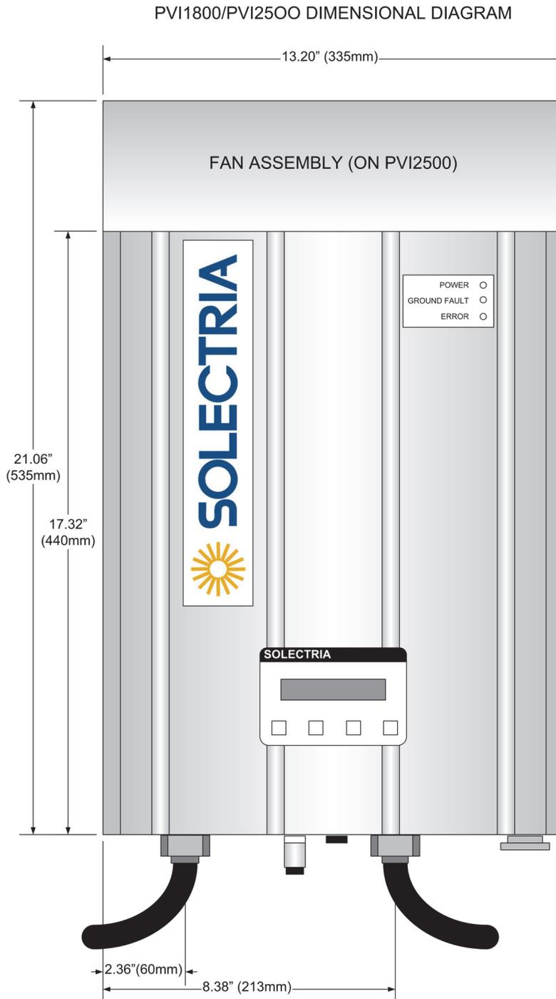
**Fig. 4 PVI 1800/PVI 2500 Dimensional Diagram**
