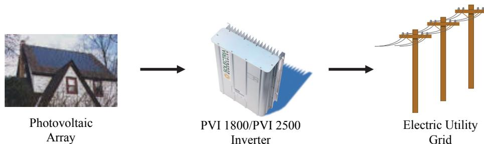
**Fig. 1 Grid tied inverter application**
