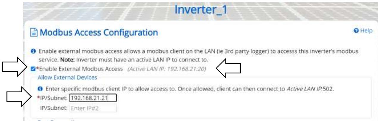
Figure 3-29 Enabling external Modbus access, static routing
