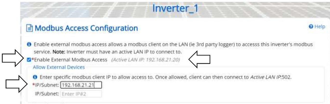
Figure 3-28 Enabling external Modbus access, Port Forwarding
