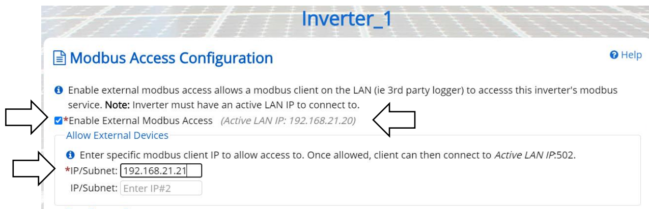
Figure 5-6 Enabling external Modbus access, Port Forwarding
