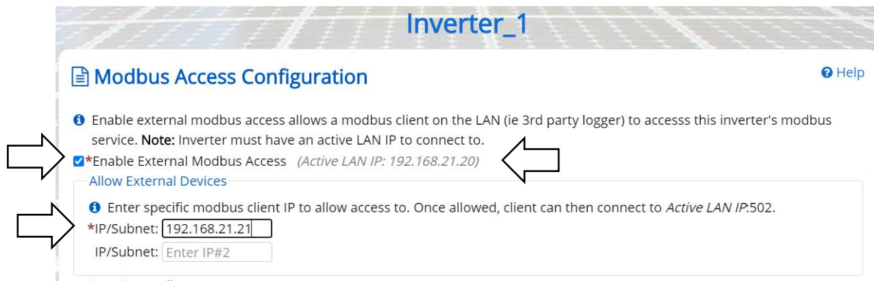
Figure 5-8 Enabling external Modbus access, static routing
