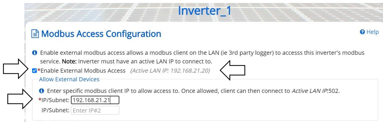
Figure 5-6 Enabling external Modbus access, Port Forwarding
