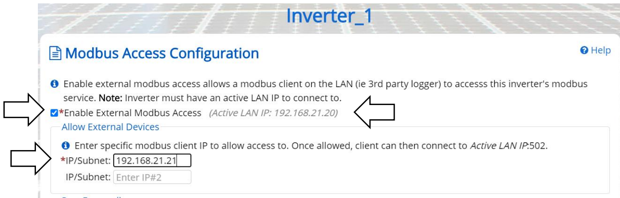
Figure 5-6 Enabling external Modbus access, Port Forwarding
