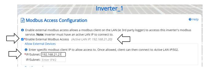
Figure 5-6 Enabling external Modbus access, Port Forwarding
