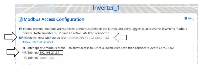
Figure 5-8 Enabling external Modbus access, static routing
