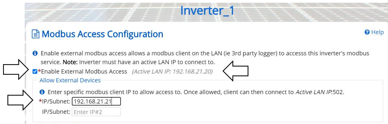
Figure 5-8 Enabling external Modbus access, static routing
