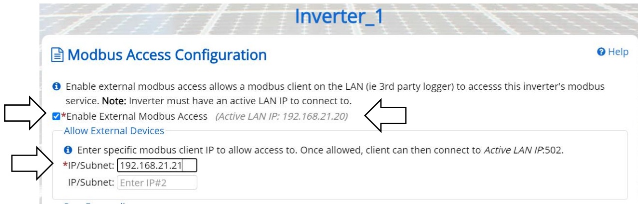
Figure 5-6 Enabling external Modbus access, Port Forwarding
