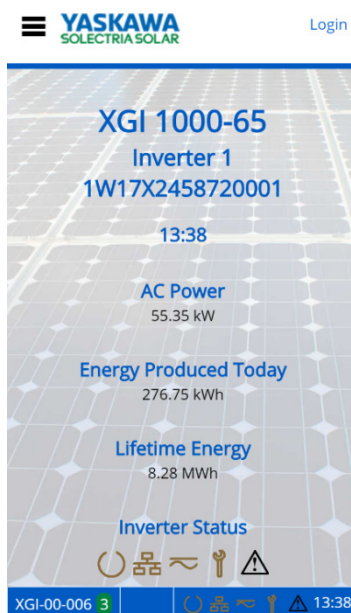
Figure 6-2 Inverter Home Page (Observer Mode)
