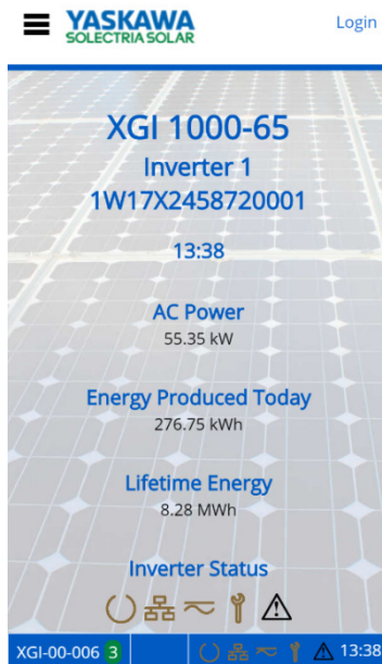
Figure 6-2 Inverter Home Page (Observer Mode)
