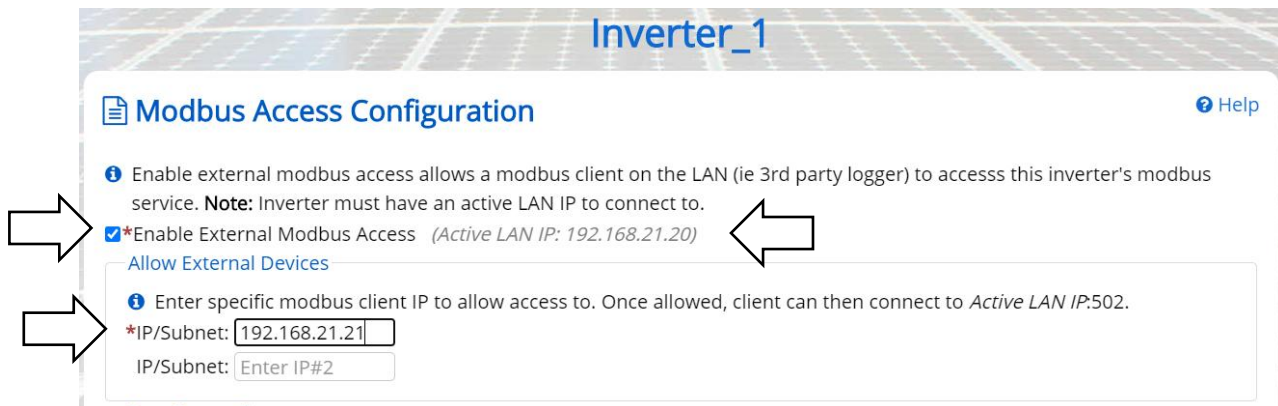
Figure 5-6 Enabling external Modbus access, Port Forwarding
