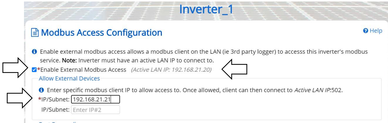
Figure 5-8 Enabling external Modbus access, static routing
