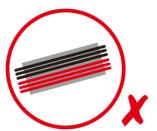
Do not separate PV + and PV - in a cable tray
