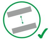
The cable trays for two different rapid shutdown systems should be installed as far apart as possible
